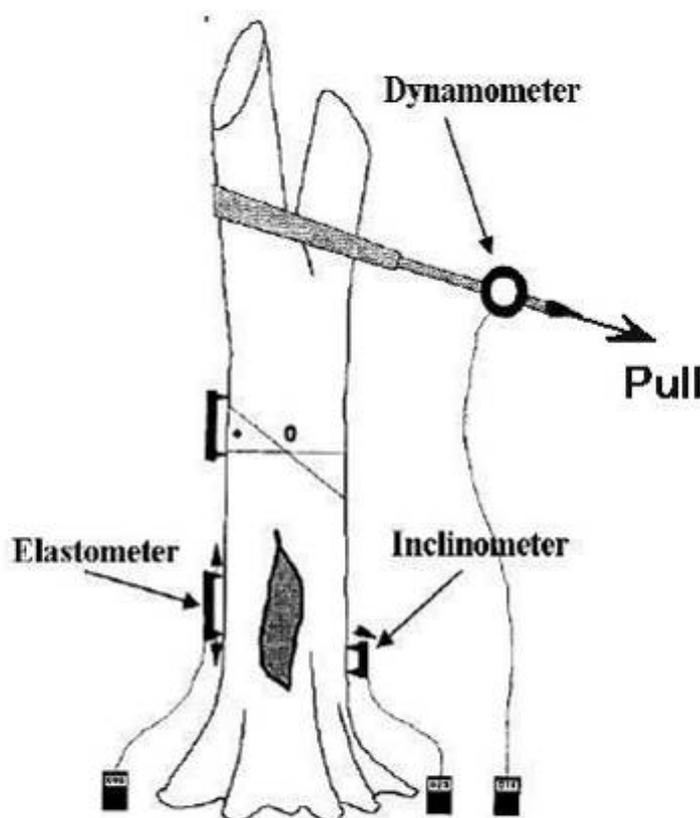
An illustration of a Pull Test
